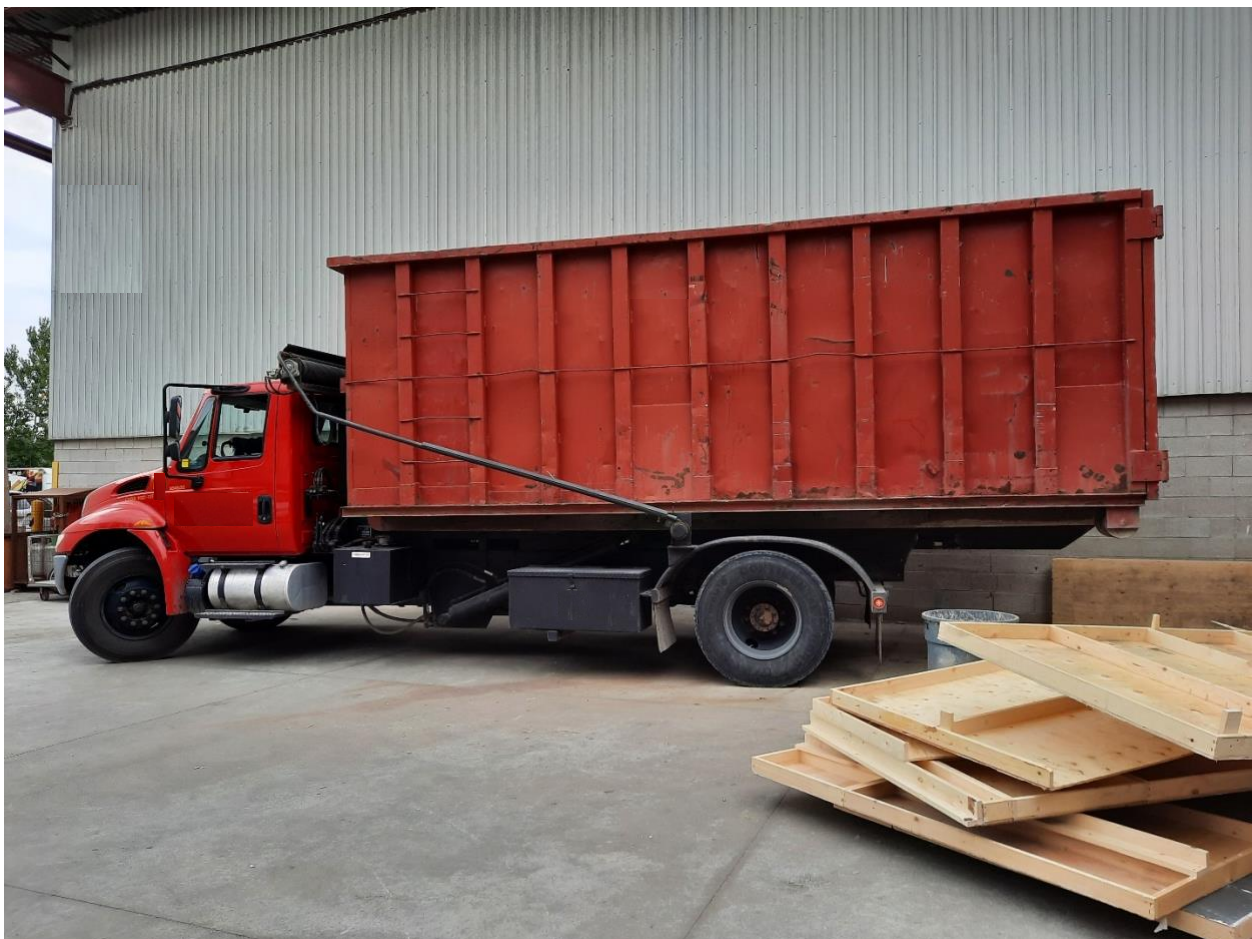
Image of a truck collecting a roll-off construction waste bin. Photo taken by Samantha Leigh, Green Spark Group.
